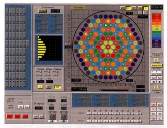
shown as a single loop. Four steam generators are individually modelled. Reactivity control has a separate screen that shows the limit control diagrams and the status of the three reactivity control devices that are under the control of the reactor regulating system.
