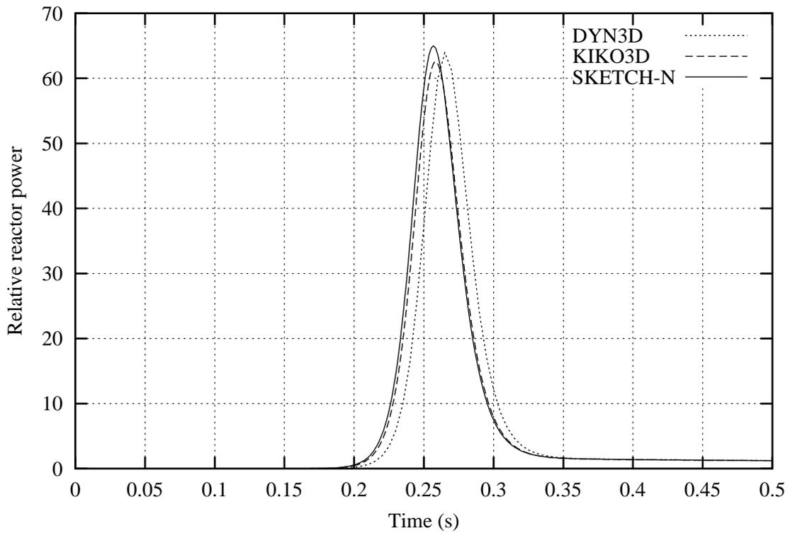
Figure 10: Reactor power vs. time,  $\Delta\rho_{\text{SKETCH-N}} \approx \Delta\rho_{\text{DYN3D}}$
