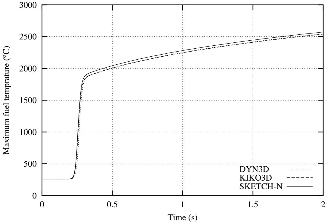
Figure 11: Maximum fuel temperature vs. time  $\Delta\rho_{\text{SKETCH-N}} \approx \Delta\rho_{\text{DYN3D}}$
