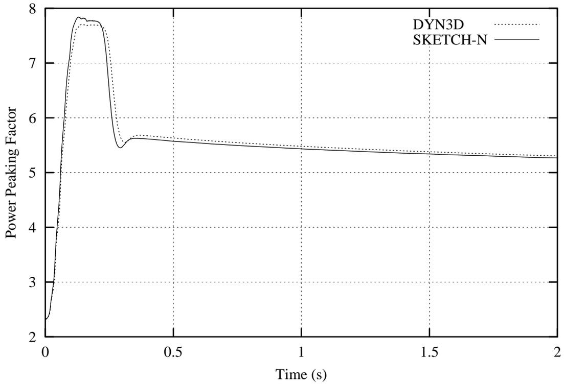
Figure 9: Power peaking factor vs. time
