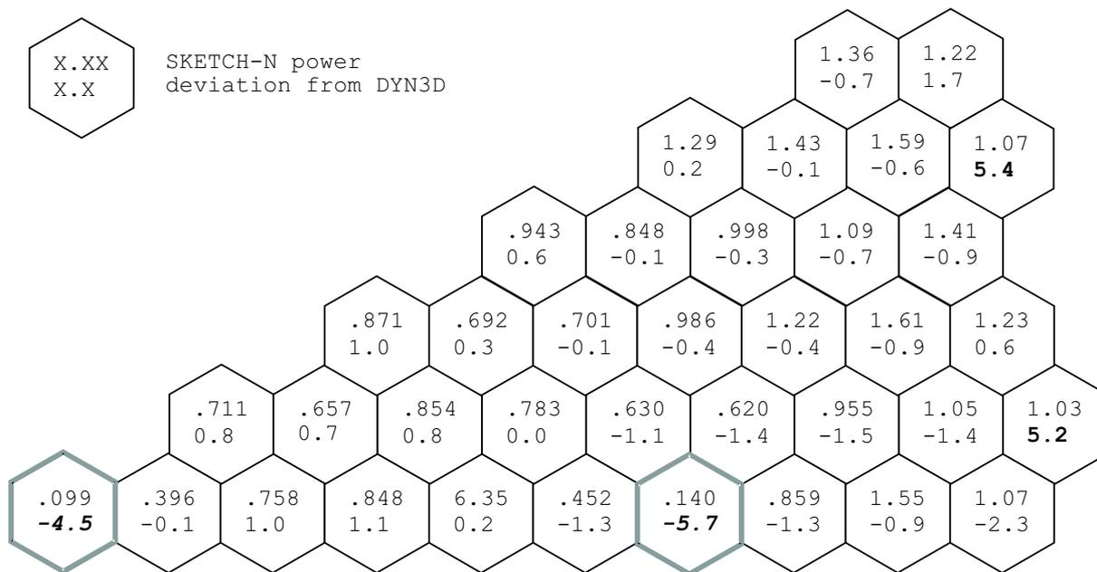
Figure 1: Assembly power of the SKETCH-N code and the deviations from the DYN3D results
