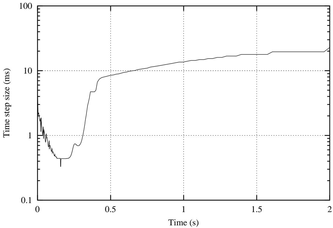
Figure 4: Time step size of the SKETCH-N code
