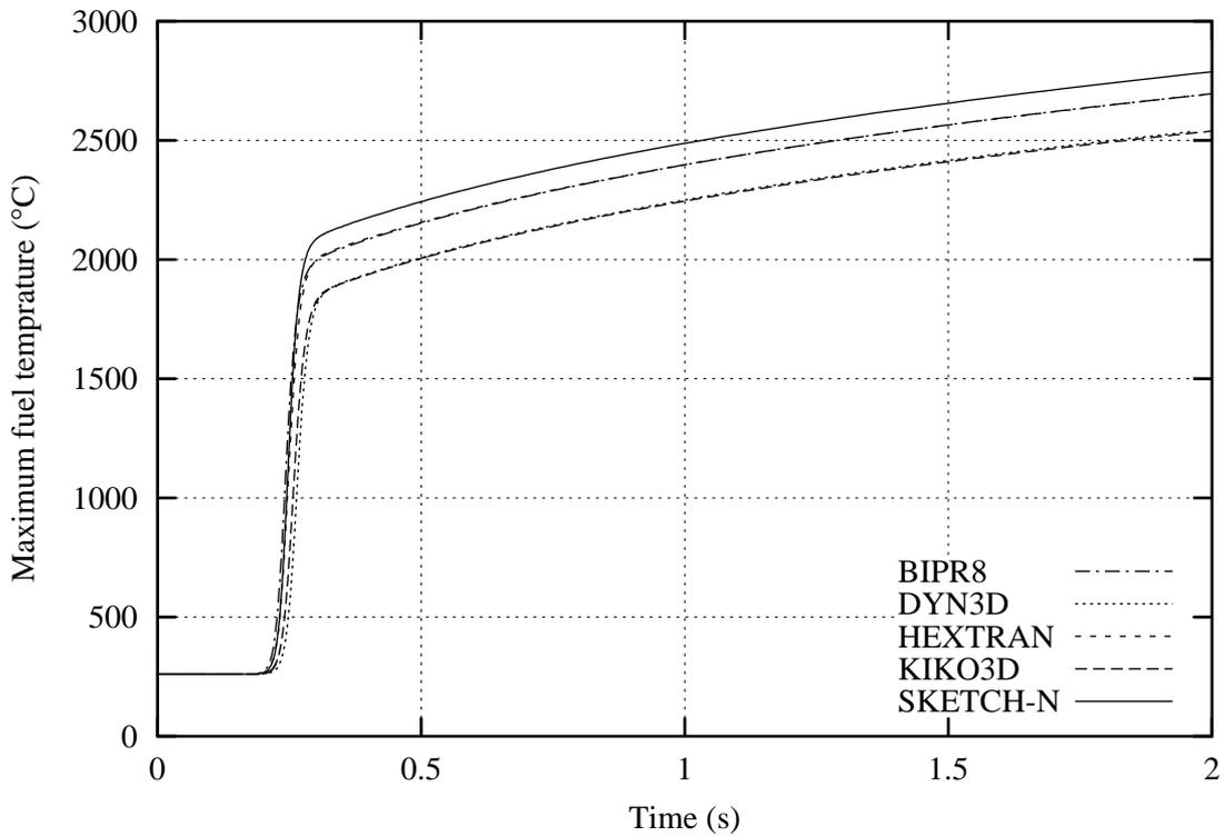
Figure 8: Maximum fuel temperature vs. time
