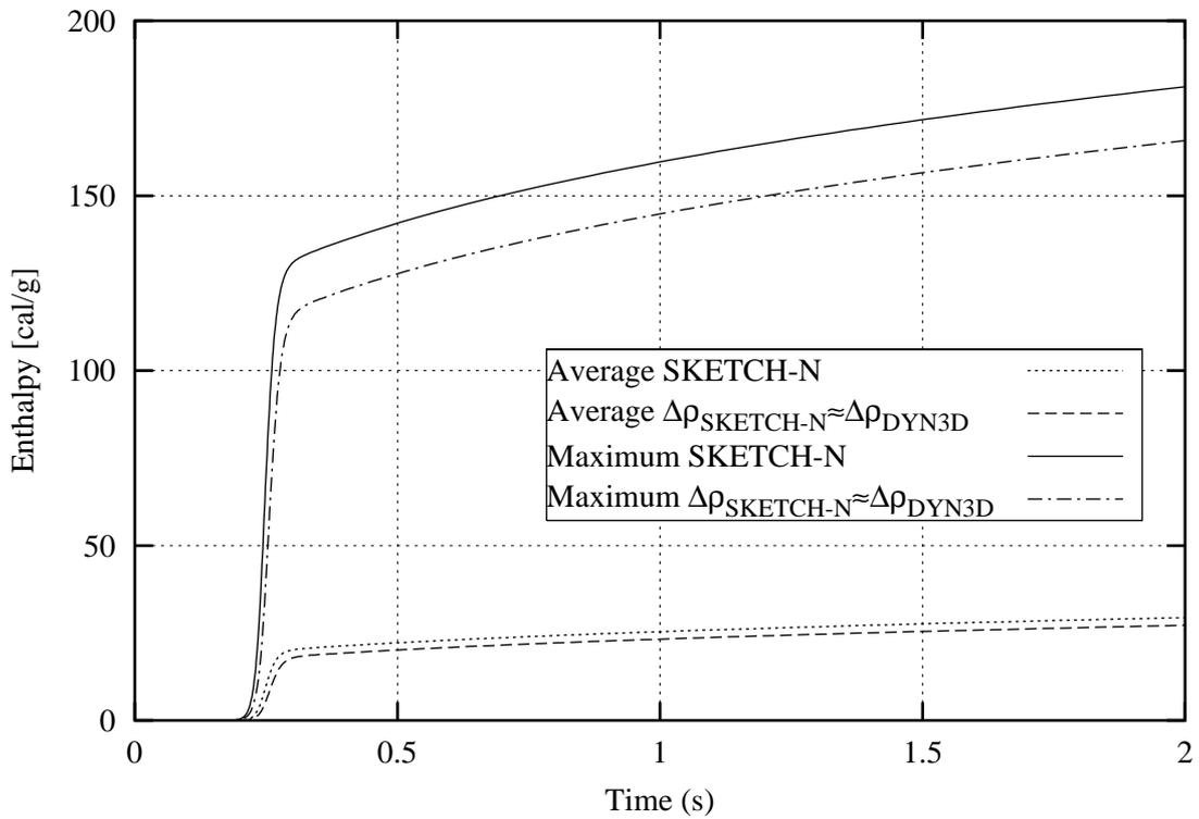
Figure 12: Reactor-averaged and maximum enthalpy injected into the fuel
