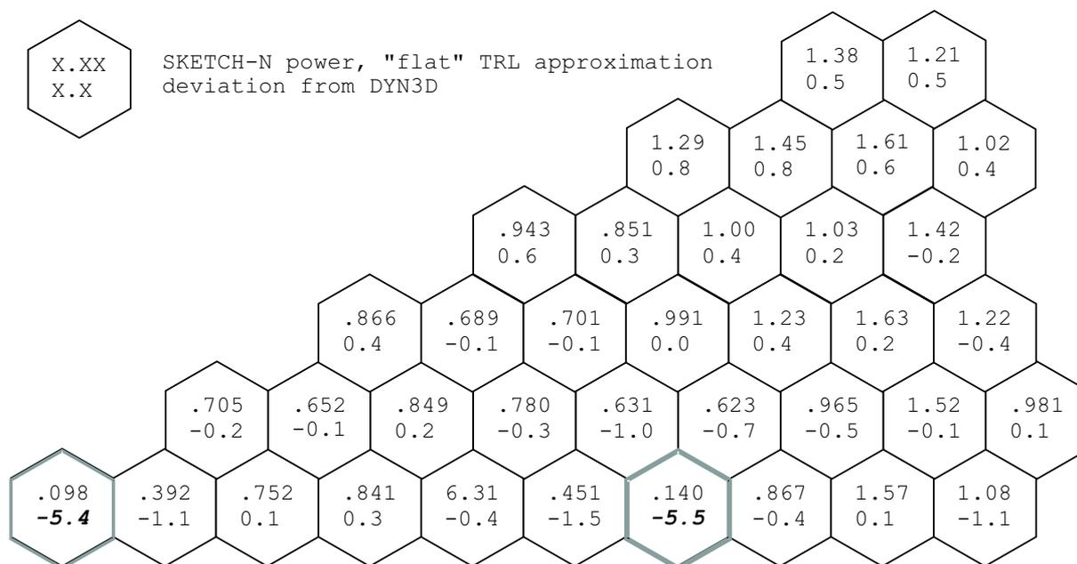
Figure 2: Assembly power of the SKETCH-N code using "flat" transverse leakage approximation and the deviations from the DYN3D results
