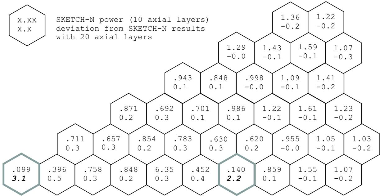
Figure 3: Assembly power of the SKETCH-N code (axial mesh size 25 cm) and the deviations from the SKETCH-N results with the axial mesh size of 12.5 cm
